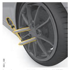
Screw in two assembly aids on vehicles with PCCB
