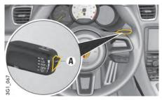
Switch for rain sensor sensitivity (A)
