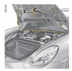
3. retaining strap B on the underside of the plastic cover and attach to the luggage compartment lid.
