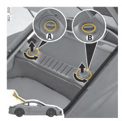
**A** - Topping up coolant **B** - Topping up engine oil
