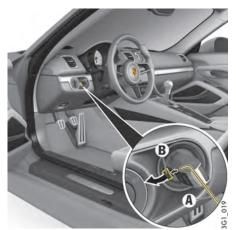
3. Use metal hook A to remove the plastic cover **B** from the ignition lock. Make sure not to lose the plastic cover **B**.
