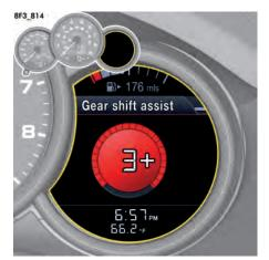
When all the segments are filled in red, a "+" sign appears next to the engaged gear in the display as a prompt to shift to the next-higher gear.
