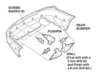
11. Using a file, remove any burrs from all holes.
