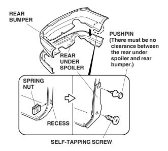
7. Using a pushpin, mark both ends of the rear bumper at the upper hole position of the rear under spoiler. There must be no clearance between the rear under spoiler and rear bumper. Remove the rear under spoiler.
