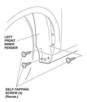
3. Position the left front splash guard on the left front inner fender, and reinstall the three self-tapping screws you removed. Tighten the three self-tapping screws in the order shown.
