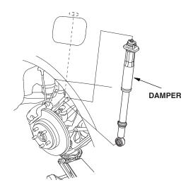
26. Compress the damper by hand, and move it into position.
