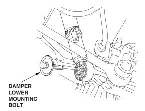
28. Loosely install the flange nuts.
