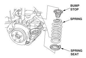
38. Install the bump stop, spring, and lower spring seat.
