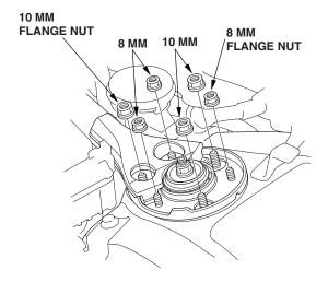
10. Install the damper fork over the driveshaft and onto the lower arm while pushing the lower arm down. Install the front damper in the damper fork so the aligning tab is aligned with the slot in the damper fork.
