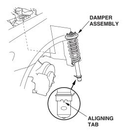
9. Loosely install the 8 mm flange nuts and the 10 mm flange nuts on the top of the damper.
