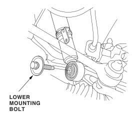
25. Remove the damper from the vehicle.
