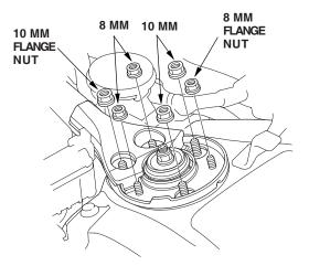
7. Remove the front damper assembly.
