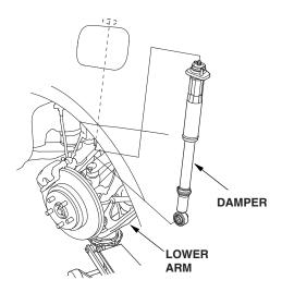
27. Loosely tighten the damper lower mounting bolt.
