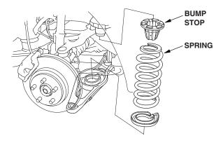
39. Align the bottom of the spring, the stepped part of the lower spring seat, and the lower arm.
