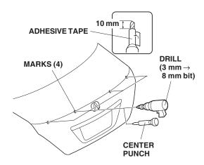
15. Remove the marking tape from the inside of the trunk spoiler.
