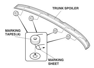
8. Remove the other adhesive backing from the four marking tapes. Do not remove the yellow tape adhesive backing.
