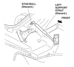
33. Install the new stud ball on the trunk hinge arm. Tightening torque: 10 N·m (8 lb-ft).
