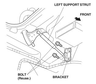
32. With an assistant holding the trunk lid, remove the support strut by removing the stud ball. Open the trunk lid halfway to facilitate removal of the stud ball.
