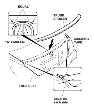
7. Remove the marking tapes from the marking tape sheets, and attach one marking tape over each threaded hole on the spoiler.
