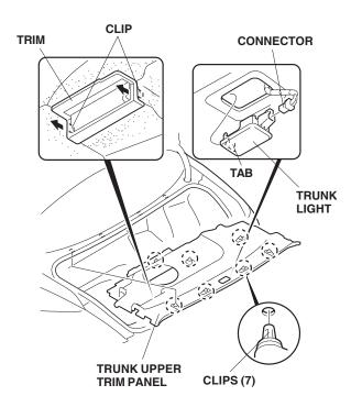
30. Remove the trunk upper trim panel (seven clips and two clips on the trim).
