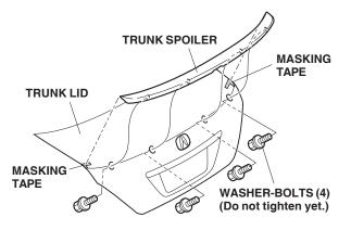
21. When the trunk spoiler is aligned properly with the trunk lid, carefully remove the adhesive backing on each side. After removal of the adhesive backings, apply sufficient pressure to the entire surface.
